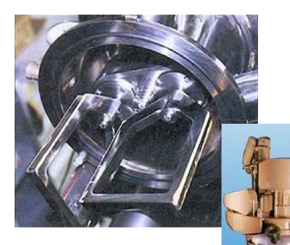
Planetary mixers are used for highly viscous material for mixing in paste form. The mixing Unit assembly rotates with a Planetary Motion contains two sets of Blades viz one set of blade rotates as well as revolves and the other blade sweeps the entire circumference of the container.
